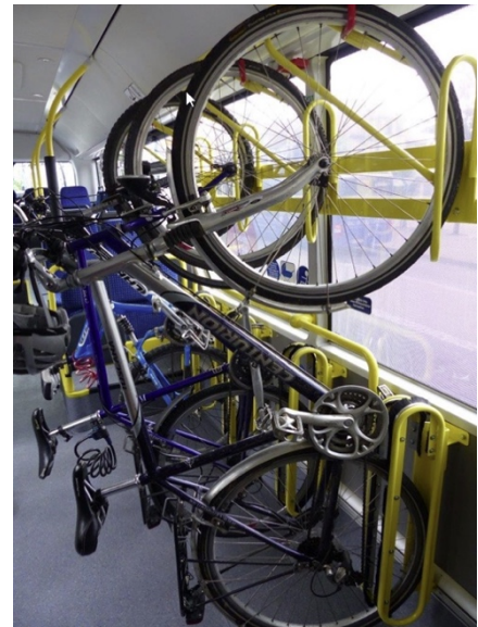
Figure 2. Improved bicycle transport through the project Fahrrad2Go. Brackets inside buses. Image courtesy of VVS.
