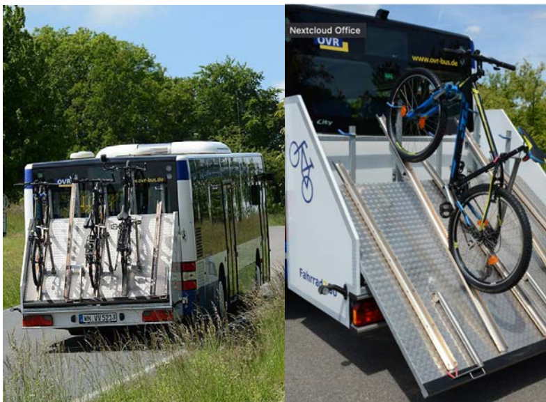
Figure 1. Improved bicycle transport through project Fahrrad2Go. Special bracket for the rear of standard buses. Image courtesy of VVS.
